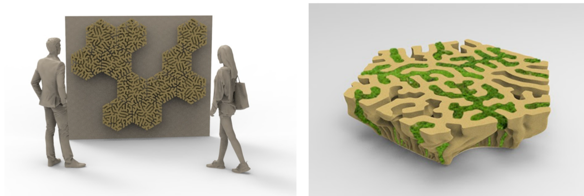
Figure 5: Digital approximation of the installation and render of the printed module with moss in it
